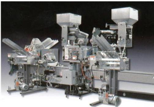
One or more Batchmaster® Counters or Fast Automatic Weighers can be used to fill a wide variety of items into clamshell packages. Typical applications include hardware and fasteners such as those seen on the shelves at your local home improvement store. Drop into the clamshell is primarily random, however magnetic orientation is available for long metallic parts such as nails and screws.
