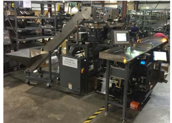
Dual Batchmaster® Counter and Hand Feed Stations
