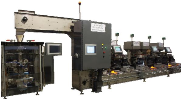
Kit Packaging System with Counters, Bagger, and Conveyor
